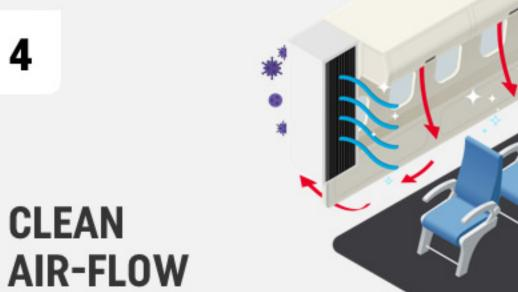
The systems our aircraft equipped with release **the clean air inside the cabin** through air vents and withdraw it from the lower part of the cabin, sending it to HEPA filters and outside. Thus, the air inside the cabin does not travel horizontally between the seats.
